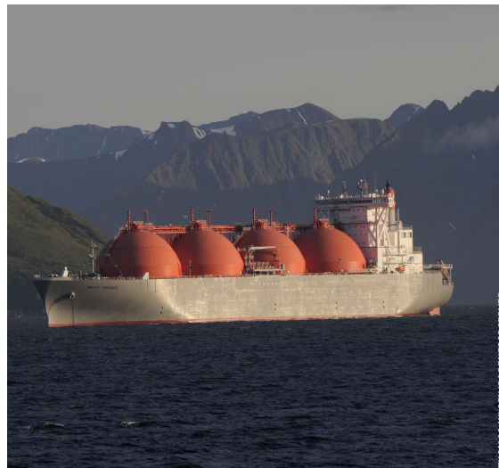
Tanker for liquefied natural gas (LNG) outside Hammerfest in northern Norway
